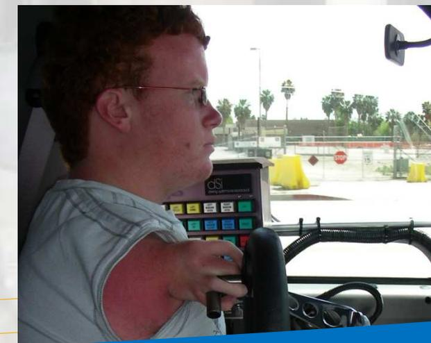
All essential driving controls are brought to a single vertical control column. Forward movement of the column opens the throttle providing control of power from the engine. Returning the control column to neutral returns the throttle to idle position. Movement of the column toward the rear applies the vehicle brakes in proportion to the pressure applied to the column.
