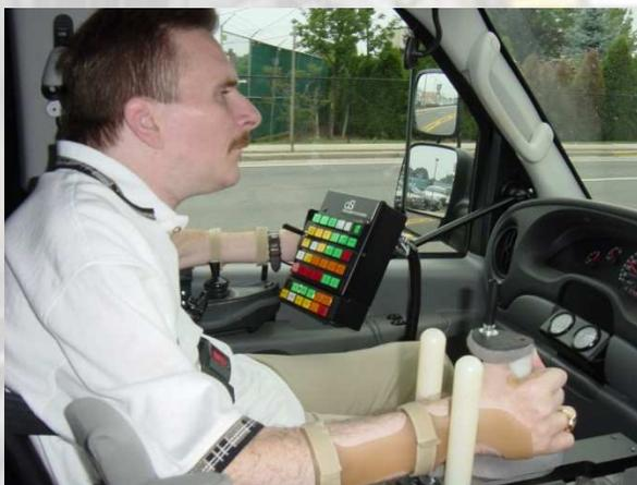
For persons who do not have finger dexterity or wrist function, such as high-level spinal cord injury, a Tri-Pin device mounted at the top of the vertical column with a parallel arm support provided.
